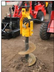
Earth drill installation
